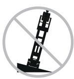
Models with outriggers: Do not lower the outriggers unless the machine is on a firm surface. Avoid drop-offs, holes, unstable or slippery surfaces and other possible hazardous conditions.
