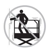
Do not push off or pull toward any object outside of the platform. Do not place or attach fixed or overhanging loads to any part of this machine.
